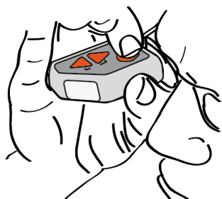
HOLD THE EC II-R INSTRUMENT WITH THE BUTTON OVERLAY FACING UPWARDS WHEN MEASURING ANGLES AND HEIGHTS.
