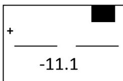
Measure the angle to the lower part of the measuring object by aiming with the two horizontal lines in the display. Press the button.
