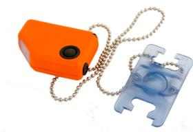
**The HEC-R** offers accurate height results from any known distance. Use the built-in basal area functions to count number of stems in your HEC-R, using one out of four basal area factors (0.5,1,2,4 or 5,10,20,40). The HEC-R will automatically display a calculation of the basal area. One dominant tree height will be used to calculate volume/ha. Measure in m/deg; m/% or ft/deg, ft/% (factory set).
